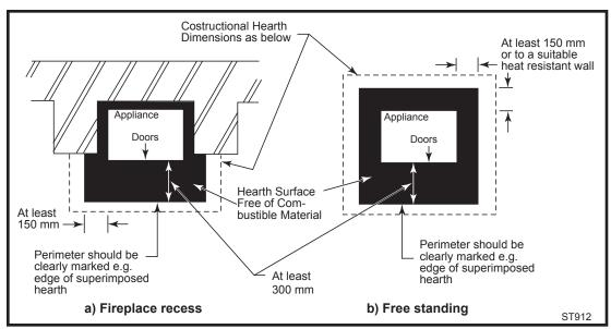
Fig. 10 Noncombustible hearth surface dimensions.
